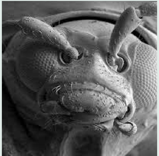
Image: Scanning electron microscope produces close-up detail, but the process is expensive, time consuming, may damage the specimen, and is generally not suitable for soft tissue specimens.
